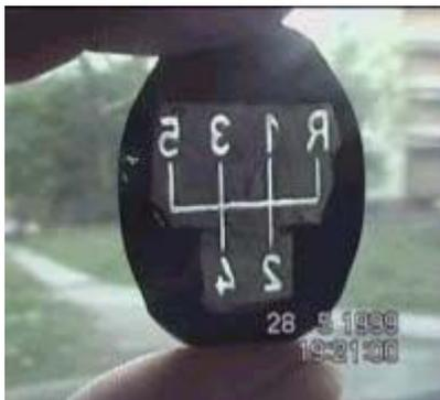
On the back of that thing you will see engraved digits, R and the directions of the gears. They are covered by light paint like the rest of the back side of plastic cover. I took a needle (you can use any sharp thin thing) and eliminated the paint only from the digits and direction lines, so they became clear (Fig. 2).
