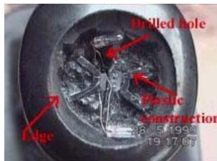
As you could notice, there is no room for bulbs under the plastic cover. I used a sharp knife to make some room. I cut out the rubber-like material until I reached the plastic construction of the knob. You have to leave the edge so the plastic cover could rest on it. It looked like this:
